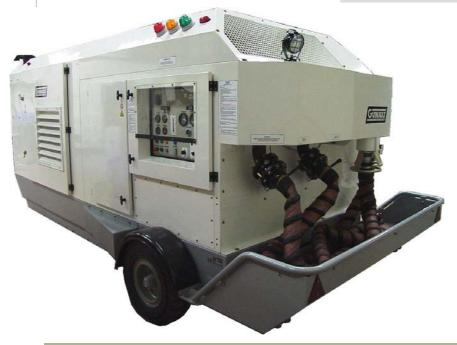
**⇒** Exclusive engine speed regulation (1300 – 1850 rpm) depending on aircraft air flow requirements
