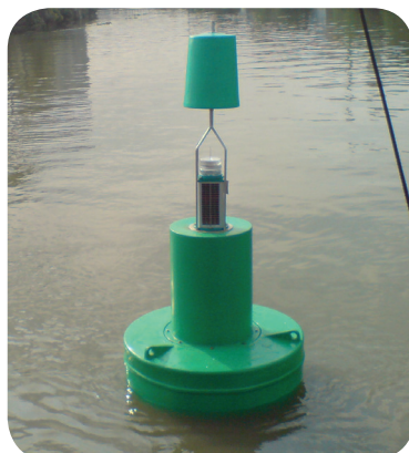
SLC420's mounted on SLB1250 Navigation Buoys, Pasig River, Manila, Philippines
